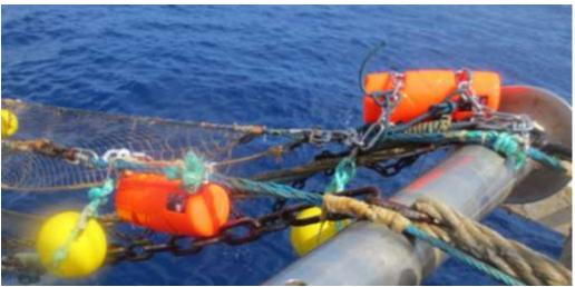
In addition, a TD probe (DST centi Star:Oddi) was placed on the net to record bottom temperature.
