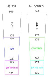
Scheme of the nets used during the experimentation. Extension piece and codend.
