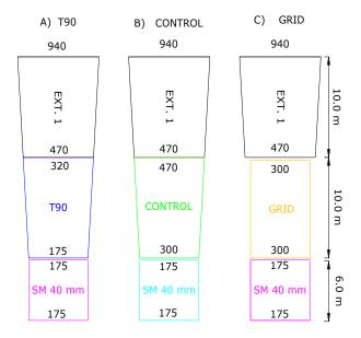
Scheme of the nets used during the experimentation. Extension piece and codend.
