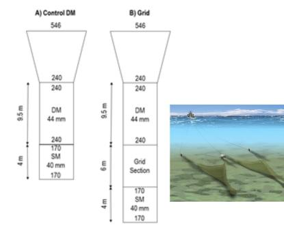
Scheme of the nets used during the experimentation. Extension piece and codend.
